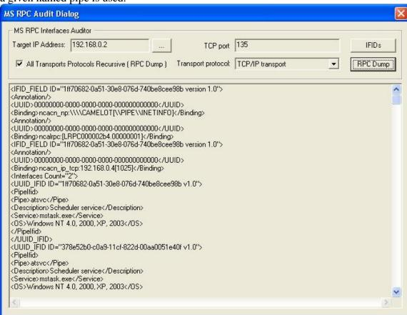
Enter the **Target IP Address** by clicking on the **Browse** button and select the **Transport Protocol** from the combobox.
